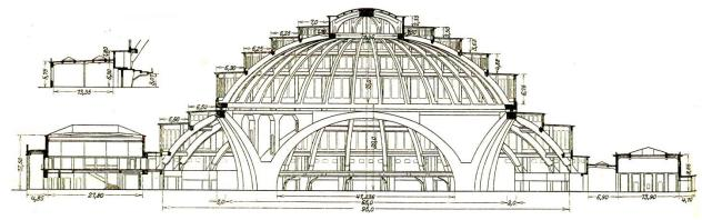
Figure 1: Cross section of Centennial Hall in Breslau (Trauer/Gehler 1913 & 1914)
