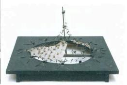
Figure 4-6: *Institut für Leichte Flächentragwerke* Stuttgart, IL-Pavillon 1966-1967, form-finding soap-film model, physical model 1965 double-exposure shot, the preserved model 2012 (IL 18, p. 477/saai Karlsruhe/DAM Frankfurt)
