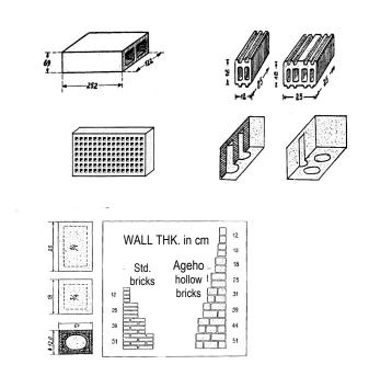
Figure 1: Five different types of hollow/perforated clay brick
