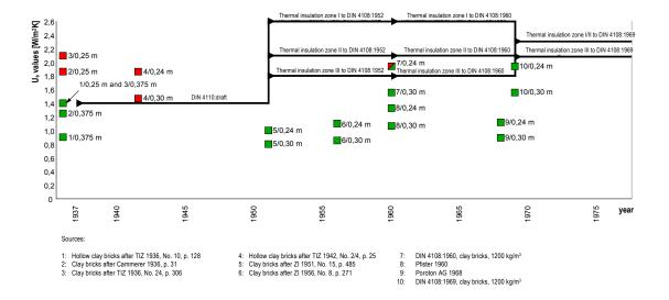
Figure 3: Comparison of requirements in standards regarding thermal transmittance and the thermal transmittance values of clay bricks for given wall thicknesses, determined according to  $U \approx \lambda/d$  and plotted against time
