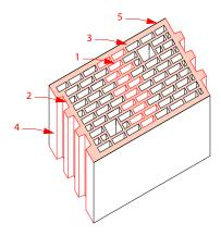
Figure 5: Five features of clay bricks: 1) offset webs and voids, 2) tongue and groove perpends, 3) fine pores, 4) parallel bed joints, 5) large block format
