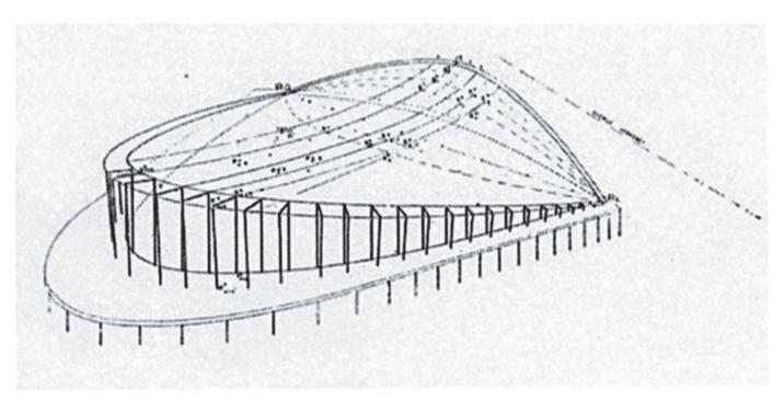
Fig. 2: Unrealised project (1951) by Laffaille for roofing the CIM (Centre of the Mechanical Industries) with a steel membrane or steel cables (Nogue, 2004, 195).
